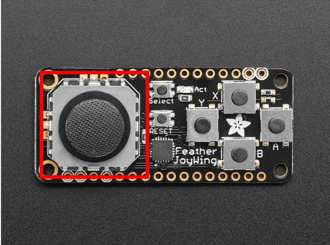
Provide a tuple of (x, y) to set your joystick center to (0, 0). The offset you provide is subtracted from the current reading. For example, if your joystick reads as (-4, 0), you would enter (-4, 0) as the offset. The code will subtract -4 from -4, and 0 from 0, returning (0, 0).
