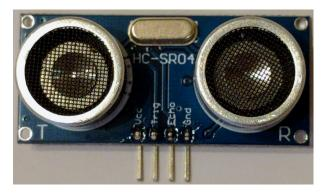
The HC-SR04 is an inexpensive solution for measuring distances using microcontrollers. This library provides a simple driver for controlling these sensors from CircuitPython.
