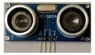
The HC-SR04 is an inexpensive solution for measuring distances using microcontrollers. This library provides a simple driver for controlling these sensors from CircuitPython.
