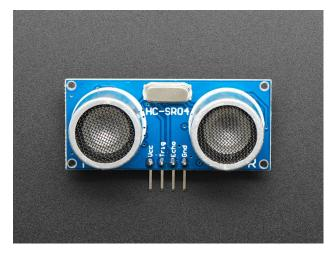
The HC-SR04 is an inexpensive solution for measuring distances using microcontrollers. This library provides a simple driver for controlling these sensors from CircuitPython.
